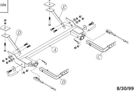
**IMPORTANT:** All brackets **must** be assembled with all the bolts left loose for final adjustment and positioning (before tightening) unless otherwise instructed. All bolts *must* be torqued for proper strength. If more than one bolt is used per fastening point, the diagram may only show one.
