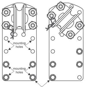
Use any of the eight mounting holes for the four self-tapping screws, based on the application.
