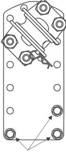
A minimum of three selftapping screws must be used.
