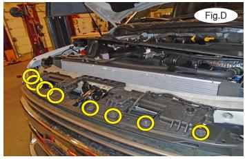
1. Important: please use all supplied bolts and parts and read all instructions carefully before beginning this installation. The majority of questions you may have can be answered within the text, and proper installation will ensure safe and secure travel. If you do not have ACC (Automatic Cruise Control), skip to step 8. Now, begin the installation. Remove 14 plastic fasteners attaching the radiator cover to the core support (Fig.C).
