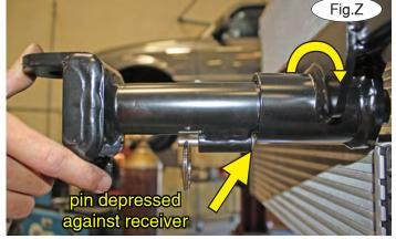
22. On each side, insert the removable front bracket arm into the front receiver 90 degrees from its final towing position, depressing the spring-loaded pin against the receiver (Fig.Z). Now, twist back 90 degrees until the spring-loaded pin snaps into place in the notch on the receiver, locking the arm into place in its final towing position (Fig.AA).
