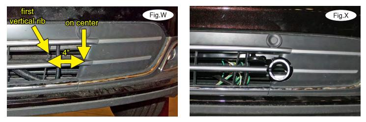
17. Hold the fascia in place over the main receiver brace. On each side, locate the first vertical rib and measure 4" toward the outside of the vehicle, mark on center in the center of the middle rib and cut a hole approximately 2" in diameter to allow clearance for the receiver (Fig.W and Fig.X).
