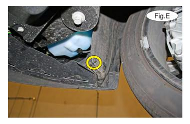
3. On each side, remove one 8mm (head) bolt attaching the fender liner to the splash shield (Fig.E). Then, remove five plastic fasteners attaching the splash shield to the core support (Fig.F).
