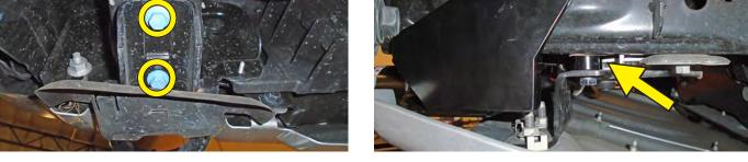
3. On each side, remove two 15mm (head) bolts attaching the tow hook to the frame and pull off the cover (Fig.C).
