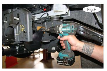
6. Working on one side at a time, position the main receiver brace below the frame rail, aligning it with the existing tow hook mount holes in the frame rail. Then, using one of the supplied  $\frac{1}{2}$ " x  $3\frac{1}{2}$ " bolts and  $\frac{1}{2}$ " lock washers, thread the bolt up through the forwardmost hole of the main receiver brace and finger tighten into the smaller weld nut with rod.
