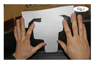
6. Locate the template at the end of these instructions. Cut out the template as shown and align it with the top profile of the lower fascia (Fig.J). Trace the template and then trim the fascia to allow clearance for the main receiver brace. *Note:* the top of the template should align as shown with the yellow lines in Figure K for best trimming results. You will also need to trim the upper edge of the lower fascia completely flat so only its mounting flange is left (Fig.L).
