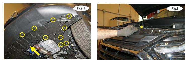
5. On each side, remove nine 7mm (head) screws attaching the lower splash shield to the subframe and fascia (Fig.H – circles), and one 7mm (head) screw in the middle (Fig.H – arrow). Remove the splash shield and set it aside for now.
