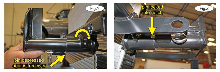
19. On each side, insert the removable front bracket arm into the front receiver 90 degrees from its final towing position, depressing the spring-loaded pin against the receiver (Fig.Y). Now, twist back 90 degrees until the spring-loaded pin snaps into place in the notch on the receiver, locking the arm into place in its final towing position (Fig.Z).
