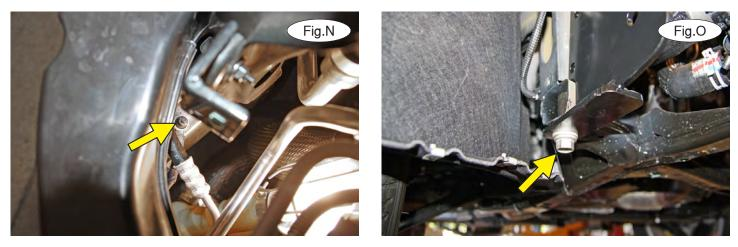
9. On the passenger side only, loosen a 10mm (head) nut and rotate the ground wire to the side to allow clearance for the main receiver brace. Re-tighten the nut (Fig.N).
