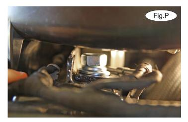
11. Place a  $\frac{1}{2}$ " flat washer over a  $\frac{1}{2}$ " x 7 $\frac{1}{2}$ " bolt, and place it through the inside mount of the rear brace. Then, place a 1 $\frac{1}{4}$ " x 1" O.D. x .188 wall pipe spacer,  $\frac{1}{2}$ " flat washer and beveled washer over the inside mount, and bolt up through the frame, finishing with the supplied beveled washer,  $\frac{1}{2}$ " flat washer,  $\frac{1}{2}$ " lock washer and  $\frac{1}{2}$ " nut (Fig.P and Q).
