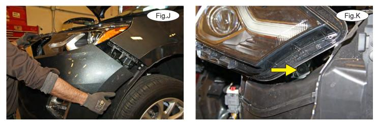
7. On each side, remove two 7mm (head) screws attaching the lower part of the headlight to the core support (Fig.K and L). Disconnect and remove the headlights, and set them aside for now.
