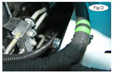
10. Place the main receiver brace under and between the frame and align it with the upper existing hole on the inside of the frame. Note: due to manufacturing variances, be sure at this point that no part of the baseplate is – or is close to – making contact with any oil or transmission coolers and their associated coolant lines.
