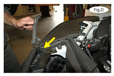
1. *Important:* please use all supplied bolts and parts and read all instructions carefully before beginning this installation. The majority of questions you may have can be answered within the text, and proper installation will ensure safe and secure travel. Now, begin the installation by removing seven T15 Torx screws attaching the top of the fascia to the core support (Fig.C). *Note:* you will need to pull off the weather stripping to expose the one on the passenger side corner (Fig.D).
