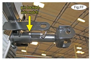
21. On each side, insert the removable front bracket arm into the front receiver 90 degrees from its final towing position, depressing the spring-loaded pin against the receiver (Fig.EE). Now, twist back 90 degrees until the spring-loaded pin snaps into place in the notch on the receiver, locking the arm into place in its final towing position (Fig.FF).
