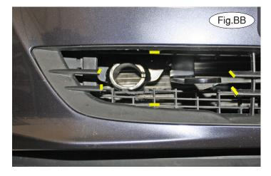
19. Reinstall the fascia, headlight and air ducting, reversing steps 1 through 6.
