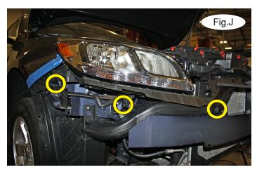
5. Remove the passenger side headlight by removing two 7mm (head) screws. Then, remove three 7mm (head) screws attaching the headlight to the frame and the air intake assembly (Fig.I and J). Unplug the headlight and remove its plastic retaining strip and set them both aside.
