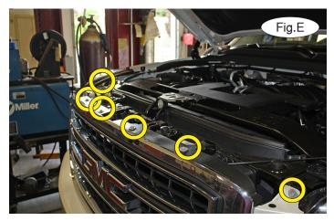
2. Remove the six innermost 10mm (head) bolts attaching the upper fascia to the core support (Fig.E).
