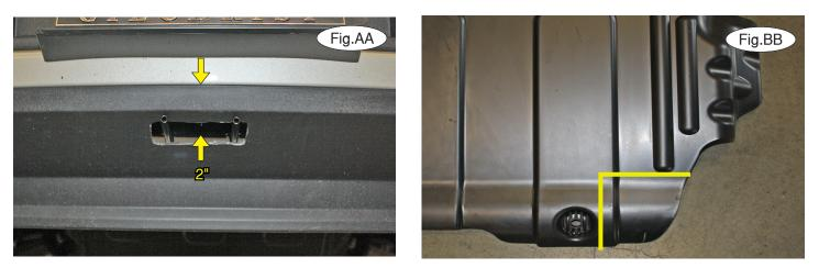
17. Looking straight on at the fascia, measure down 2" from the seam of the fascia, on center of the fascia, and trim a 1" x 4" rectangle to allow clearance for the wiring prongs (Fig.Z). Contour all holes as much as necessary to reach the desired level of detail.
