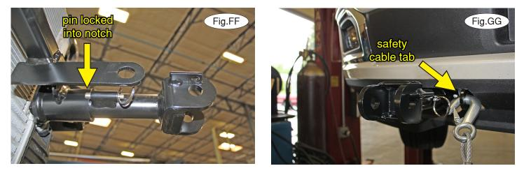
22. Install the tow bar to the mounting bracket according to the manufacturer's instructions.
