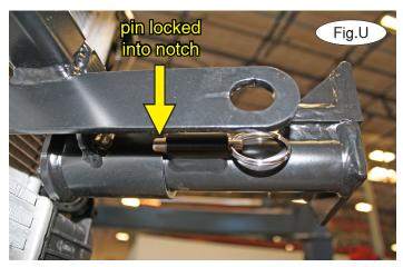
20. On each side, insert the removable front bracket arm into the front receiver 90 degrees from its final towing position, depressing the spring-loaded pin against the receiver (Fig.T). Now, twist back 90 degrees until the spring-loaded pin snaps into place in the notch on the receiver, locking the arm into place in its final towing position (Fig.U).
