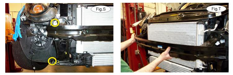
15. On each side, remove two T20 Torx bolts attaching the bumper core to the core support (Fig.S).
