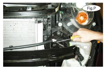
12. On each side of the radiator, remove one plastic fastener attaching the water line to the top of the bumper core (Fig.P). *Note:* due to manufacturing variances, not every vehicle will be equipped with this water line.
