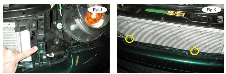
7. On each side of the radiator, remove one T25 Torx bolt (Fig.J) attaching the top of the fascia to the core support.
