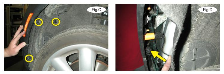
1. *Important:* please use all supplied bolts and parts and read all instructions carefully before beginning this installation. The majority of questions you may have can be answered within the text, and proper installation will ensure safe and secure travel. Now, begin the installation by removing three plastic fasteners (on each side) attaching the fender liner to the fascia (Fig.C).
