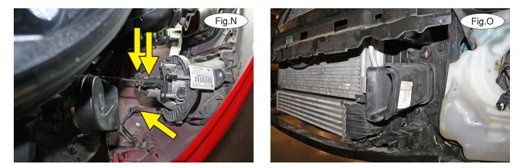
10. Pull forward on the fascia to gain access to the fog lights and disconnect them (Fig.N). Also, locate the ambient temperature sensor (on the passenger side only) and disconnect it and its wiring loom. *Note:* do not start the vehicle when the temperature sensor is unplugged because it could cause the 'Check Engine' light to illuminate.
