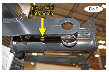
10. On each side, insert the removable front bracket arm into the front receiver 90 degrees from its final towing position, depressing the spring-loaded pin against the receiver (Fig.O). Now, twist back 90 degrees until the spring-loaded pin snaps into place in the notch on the receiver, locking the arm into place in its final towing position (Fig.P).
