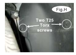
6. On the inside of the fender well there are two more T25 Torx screws that need to be removed. These are attaching the lower fender liner to the upper fender liner (Fig.H). Repeat for the other side.
