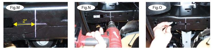
8. On each side, locate a square hole in the bottom of the frame rail. Measure 2" back from the hole, and find the center of the frame (Fig.M – passenger side).
