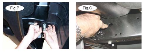
11. Hold the backing plate in place and using the bolts you removed in step 8, bolt through the rock guard, frame rail and into the backing plate (Fig.P).
