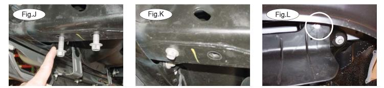
6. Now put the front bolts back in and tighten down (Fig.J), then remove the rear bolt on each side (Fig.K).
