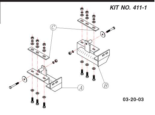
**IMPORTANT:** All brackets **must** be assembled with all the bolts left loose for final adjustment and positioning (before tightening) unless otherwise instructed. All bolts *must* be torqued for proper strength. If more than one bolt is used per fastening point, the diagram may only show one.
