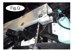
16. Now, using the two holes at the top of the main brace as templates, drill two more 17/32" holes through the bumper core (Fig.Q).
