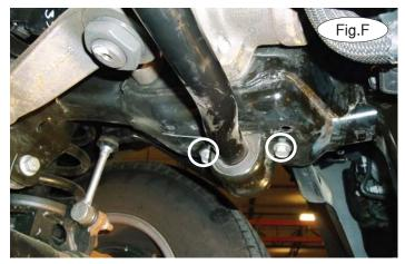
3. On each side, remove two 15mm (head) bolts attaching the sway bar clamp to the frame (Fig.F). Let the sway bar hang down for now.
