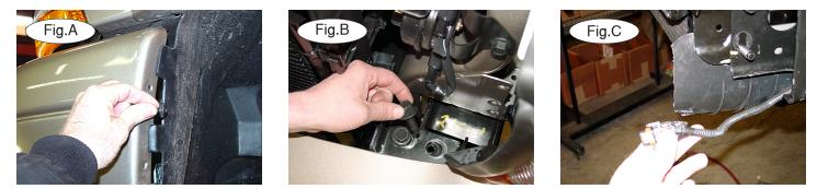
2. Remove three torx screws in each fender well (Fig. A). Disconnect the fog lights if present (Fig.B) then remove four bolts, two on the top of each frame tube (Fig.C). Now. remove two bolts on the bumper side braces on each side. These are located on the sides of the frame tubes.
