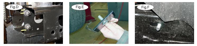
5. Working on one side at a time, locate a slotted hole about one foot back from the front of the frame. Fish wire a  $\frac{1}{2}$ " x 1<sup>1</sup>/<sub>2</sub>" carriage bolt and  $\frac{1}{4}$ " x 2" x 3" backing plate through the front of the frame into the slotted hole (Fig.E,F,).
