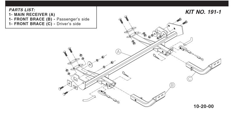
**IMPORTANT:** All brackets **must** be assembled with all the bolts left loose for final adjustment and positioning (before tightening) unless otherwise instructed. All bolts *must* be torqued for proper strength. If more than one bolt is used per fastening point, the diagram may only show one.
