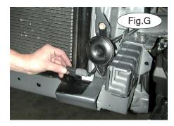
2. Remove three 10mm (head) screws on each side. One is located in the top of the fender well (Fig.D) and two are underneath on each side (Fig.E). Some vehicles may have more fasteners in the fenderwells Remove the remaining plastic fasteners in the bottom of the fascia. Pull forward on the fascia (Fig.F), disconnect the foglights (Fig.G) then set aside.
