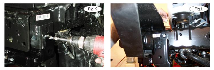
13. Using the upper outside mounting point of the main receiver brace as a template, drill a  $\frac{1}{2}$ " hole through the side of the frame support (Fig.K).
