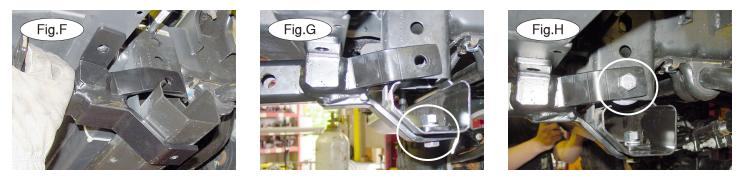
4. Beginning with the driver's side, place the driver side main receiver brace in position over the existing holes in the bottom and side of the frame rail (Fig.F).
