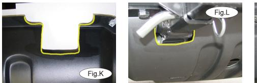
11. Refer to the yellow marker line in Figures K and L for correct trimming of the splash shield on both sides. *Note:* for trimming of the metal splash shield, refer to Figure M.
