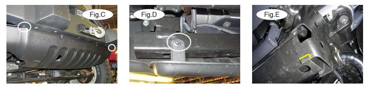
1. *Important:* please use all supplied bolts and parts and read all instructions carefully before beginning this installation. The majority of questions you may have can be answered within the text, and proper installation will ensure safe and secure travel. Now, begin the installation. Start by removing one 8mm (head) bolt from each side, detaching the splash shield from the bumper (Fig.C).
