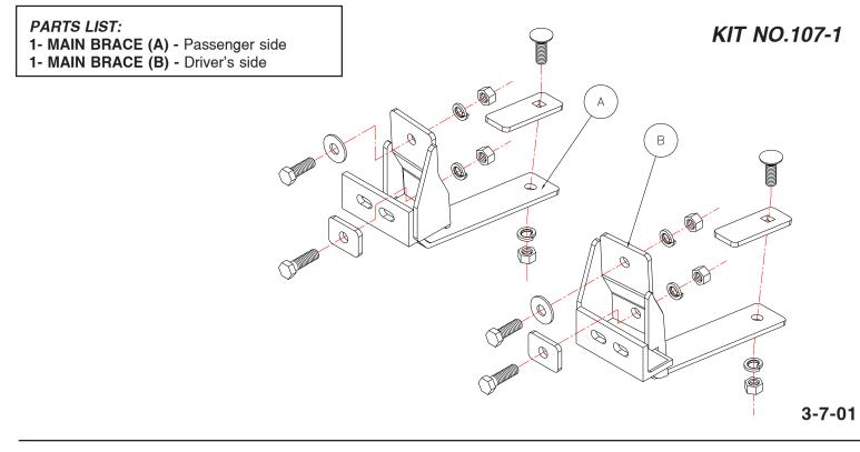
**IMPORTANT:** All brackets **must** be assembled with all the bolts left loose for final adjustment and positioning (before tightening) unless otherwise instructed. All bolts *must* be torqued for proper strength. If more than one bolt is used per fastening point, the diagram may only show one.
