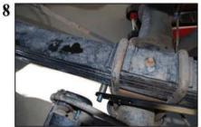
Next remove from the end hole in the Axle Conecting Bracket the nylon insert nut, tube spacer, bolt and two spacers washers (not shown in illustration (7).
