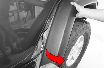
Mark the inner fender well plastic where it sticks out from the body using a pencil, sharpie or paint pen, you will be trimming the excess plastic in the next step so grab a razor blade and some shears.
