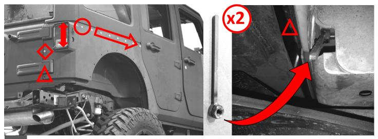
Loosely fit up the skin and begin threading one of the 3/8x1-in Button Head Bolts and Washers through the hole nearest the tail light on top where the red circle is.
