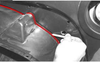
You will want to remove the plastic retainers with a panel clip pry tool like in step 2 to make trimming easier.
