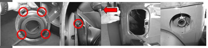
Below is the driver side top nut flange. Insert this piece through the tail light opening. Nuts will be to ward the inside of the vehicle and tab down. This step requires some forceful stabbing and sawing to get past the sprayed in foam insulation.
