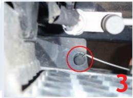
There are plastic clips behind the grill that hold in the OEM bumper in as seen in picture.
