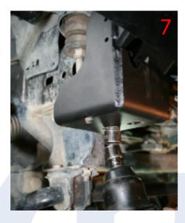
• Install the winch to the bumper using the supplied Allen Bolts and Washers. Note - Install the Flairlead bolts before you mount the winch.
