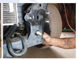
Be sure there is no powder coat on or in tube sleeves. And it may help to... um... lube it up and twist it in.
