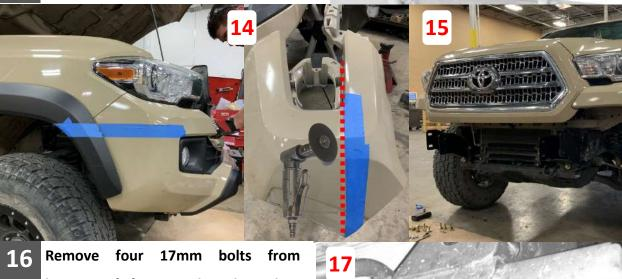
Remove four 17mm bolts from bottom of frame rail with socket.
