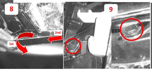
Carefully pry lose. This piece just snaps in place and will be attached to the new bracket provided.
