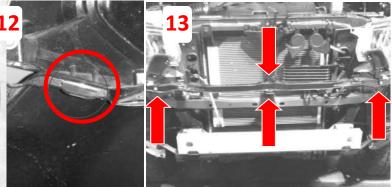
12 Remove four 10 mm nuts from center factory bumper cover support structure and set aside.
