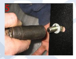
Install the winch to the bumper using the supplied Allen Bolts and Washers.
