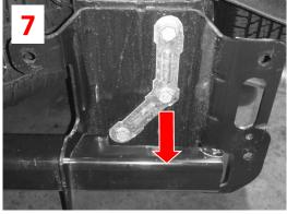
Install Road Armor bracket one side at a time using the now Double Bolt Tabs in bracket, Single Bolt Tab through lower hitch mount and the included 1/2" hardware. Outer holes may need to be drilled to 1/2", if this is necessary be sure to paint.
