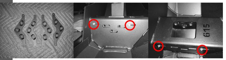
15 Measure left to right on bumper and adjust brackets to the same distance before attempting fit up.
