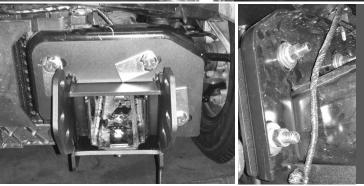
Install brackets using five (5) bolt tabs, followed by a washer, lock washer and nut. Do not tighten bolts fully, or you won't be able to adjust the bumper's fitment and will have difficulty aligning brackets to bumper.
