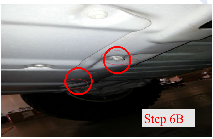
Step 6B: Remove Skid plate
