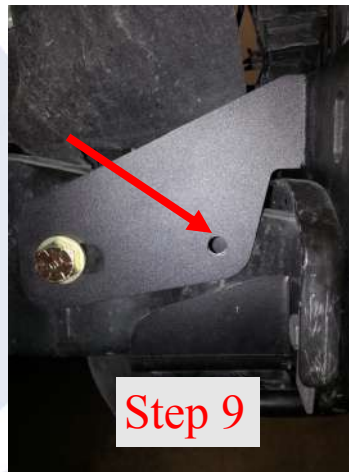
Step 9: Drill mounting hole
