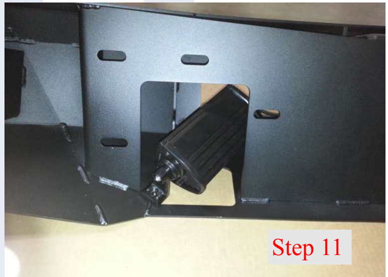
Step 11: If you are going to install center e-series lights be sure to mount them before installing the bumper
