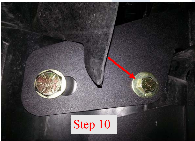
Step 10: Install 1/2" hardware
