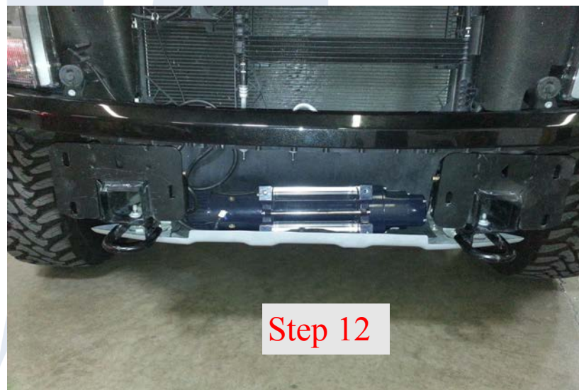
Step 12: Now re install the skid plate to your vehicle. If your going to install a winch the front lip of the skip plate is a good place to hold the winch while you are finishing up the mounting of the bumper.
