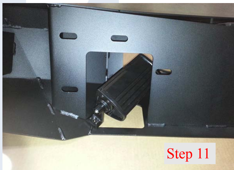
Step 11: If you are going to install center e-series lights be sure to mount them before installing the bumper
