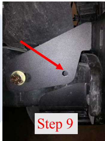
Step 9: Drill mounting hole
