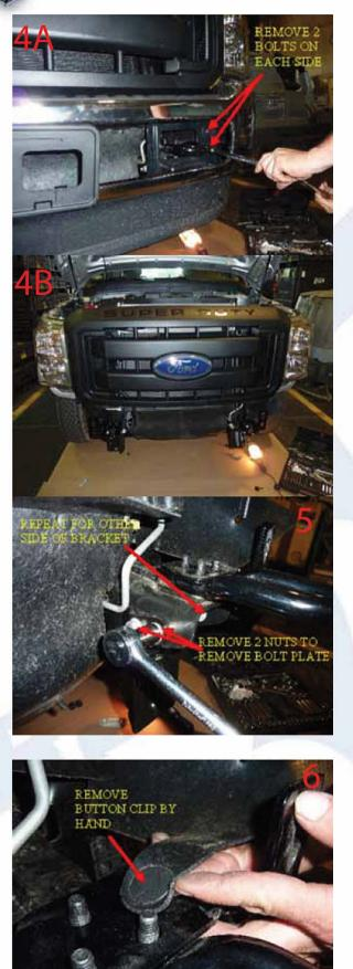
• Remove 4 nuts from the two bolt plates to remove lower frame bracket. Use a 18 mm socket to remove the nuts from the bolt plate.
