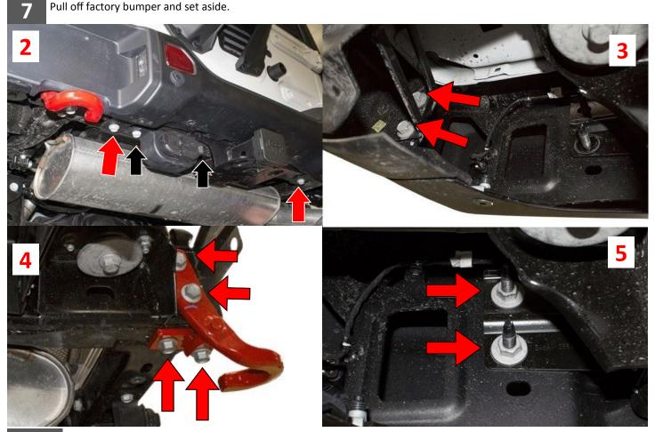
If equipped, disassemble rear bumper, carefully remove all sensors and harnesses. \*\*Note sensor location\*\*
