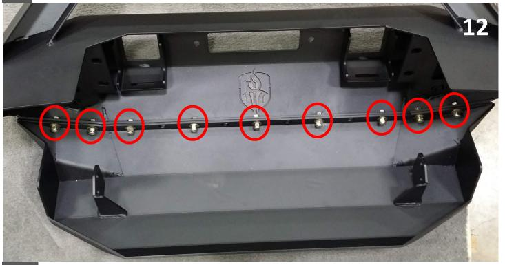
Install both cube lights, fairlead and 2 - 1/2" bolt tabs on each outer slots of bumper using retainer washers to hole install bumper using large washers on the outside
