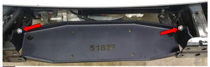
Install Road Armor Winch Plate between frame rails, using factory 12mm bolts on each side.
