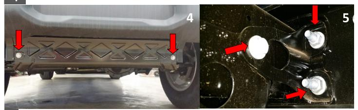
Remove the two nuts one bolt holding the factory bumper and stiffeners on, four (4) on each side of the frame using an 18mm socket and/or wrench. Keep both outside stiffeners for installing Road Armor Bumper.
