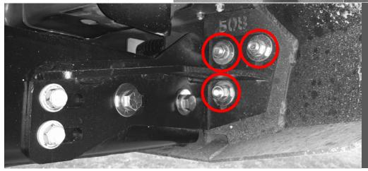
Armor Bumper and start a washer, lock washer and nut over each bolt.
