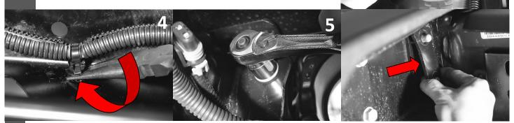
Remove the nuts holding the factory bumper on, four (4) on each side using an 18mm socket and socket wrench. Keep the backing plate for installing Road Armor Bumper.
