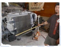
• Using a silver sharpie or paint pen mark the contour of the bumper on inner fenderwell by pulling it tight and tracing. Once traced, double check and make any necessary adjustments then cut excess plastic and tuck into bumper.
