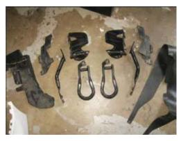
The Image on the left shows all parts that must be removed to ft Road Armor Bumper:
