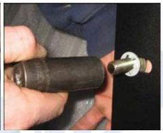
Install the winch to the bumper using the supplied Allen Bolts and Washers.
