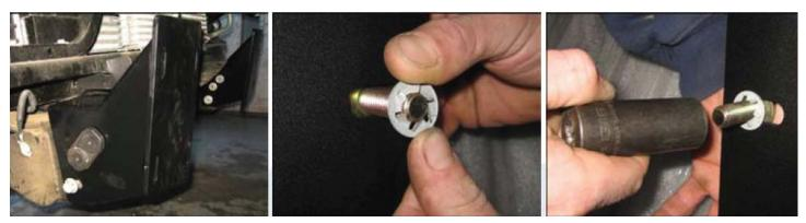
• Install the winch to the bumper using the supplied Allen Bolts and Washers. Note - Install the Flairlead bolts before you mount the winch.
