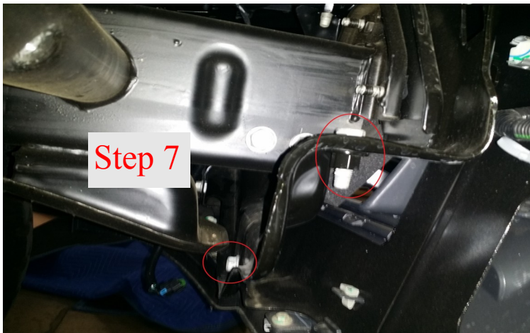
Step 7: Remove factory bumper
