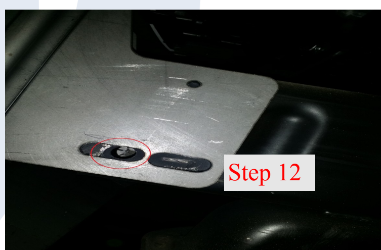
Step 12: Install bracket loosely with bolt tabs
