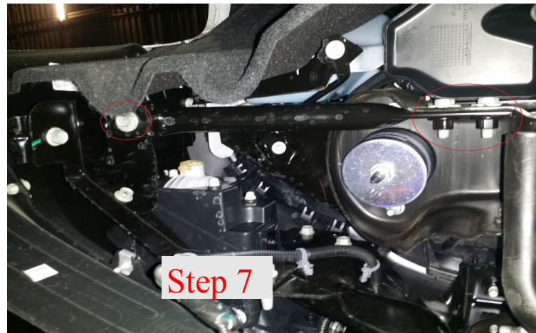
Step 7: Remove factory bumper
