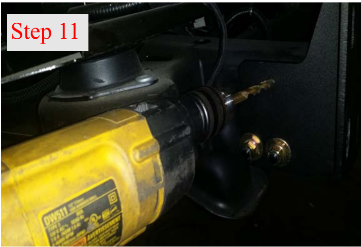
Step 11: Drill out pilot hole
