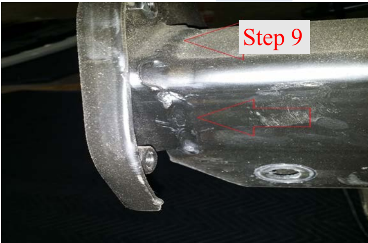
Step 11: Remove Bumper brackets and tow hook
