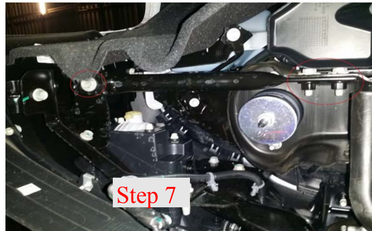
Step 7: Remove factory bumper
