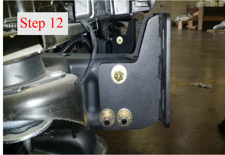
Step 12 Install mounting brackets
