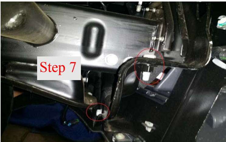
Step 7: Remove factory bumper
