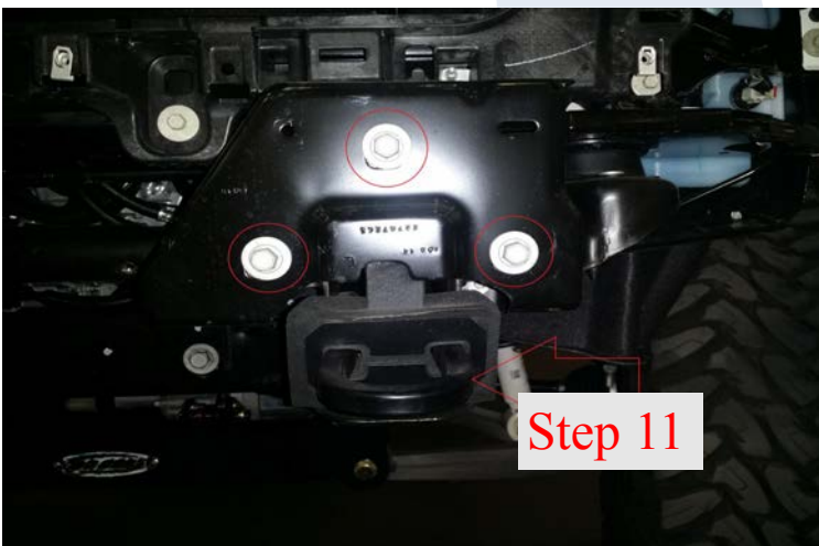
Step 11: Remove Bumper brackets and tow hook
