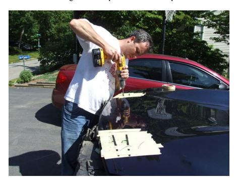
**5.** Once the holes have been drilled, remove the "T-Straps" and drill "1/4inch" holes through the top & bottom of the trunk lid.
