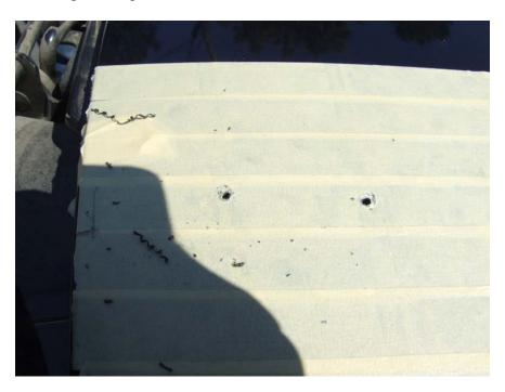
**6.** Next you will need to drill a 1" inch opening through the "INNER" portion of the trunk lid only making sure not to go through the entire trunk lid to the outer surface. This step will require a special drill bit. "Not included with spoiler".
