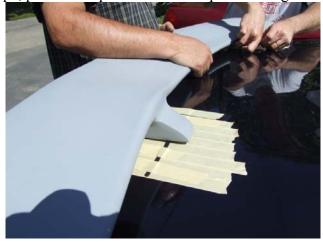
**4.** Remove the spoiler, leaving the T-straps taped to the vehicle. You will need a 1/8th" bit to drill through the TOP portion where the "pilot holes" are located.
