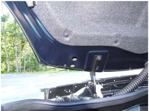
7. Using the ¼"X ¾" Pan Head Screws and the ¼"X1"inch washers, attach the spoiler.
